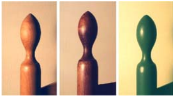
Harvard community-style back post's finials of three straight slat back chairs. Hard maple, oil finish (left). Hard maple, water-based (mahogany) wiping stain finish (center). Hard maple, oil-based paint (wild bayberry) finish (right).
